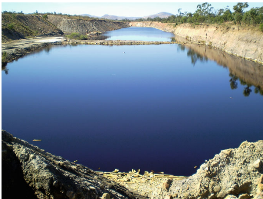
Fig. 4.7 Field macrocosms experiment at Garrick East Pit Lake (sewage and green waste treated macrocosm in the foreground, control at the back). Data: East Garrick Mine Lake: pH 2.4, sulfate 4.3–6.6 g L -1 , iron 600–650 mg L -1 , aluminum 62–110 mg L -1 (Photo: M. Lund)
