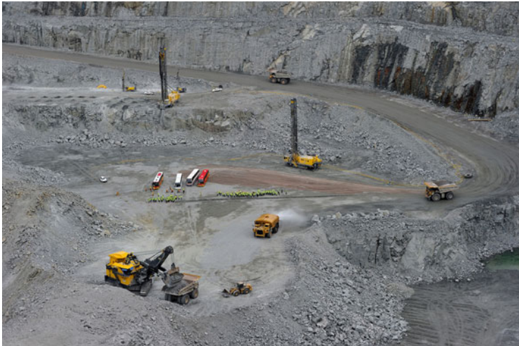
Fig. 1.2 Technology of industrial hard-rock opencast-mining. Large size excavators loading ore on giant trucks in Aitik mine/Sweden. The trucks that haul the ore can carry from 255 to 360 tons of rock. Visitors for size comparison (By courtesy of Boliden/Photographer: Daniel Olausson)
