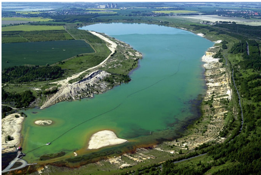
Fig. 4.4 Lake Bockwitz (central German lignite district) being treated with soda ash. The soda is delivered by tanker trucks ( lower left corner ), suspended in lake water and distributed through a 1.2 km long floating pipeline ending in the lake center ( upper right corner ; Photo: P. Radke/LMBV)
