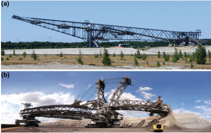
Fig. 1.1 Technology of industrial scale strip mining. a Upper photo overburden conveyor bridge (type: F60), 500 m long and 100 m high, is surpassing the size of Eifel's tower. It was used till 1992 for lignite strip mining and is shown in Lichterfeld mining museum (Lusatia, Germany; Source Lutz Bruno); b lower photo Bucket wheel (type: 288), 220 m long and 96 m high, moving 240,000 t/d of coal/overburden in Garzweiler mine/Rhenish lignite district ( Source Wikimedia commons, panorama-photo by Martinroell)
