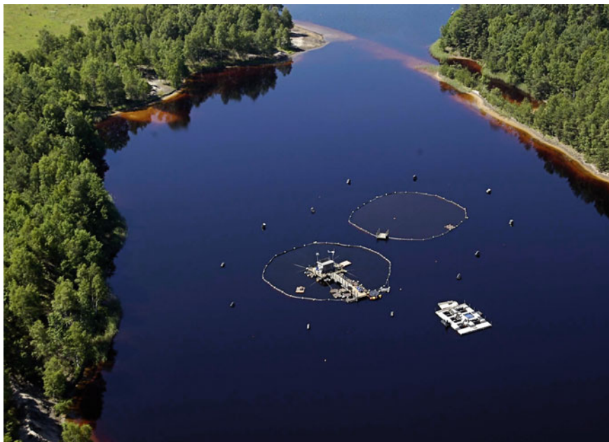
Fig. 4.6 Field experiments with enclosures of different sizes in Mine Lake 111 (Lusatian district, Germany). The smallest enclosures (about 20 m 3 ) worked successfully, but the large enclosures (4,500 m 3 ) failed to neutralize the water column because the iron sulfide formed during lake stratification were re-oxidized during the cold season with holomixis of the water (Photo: P. Radke/LMBV)
