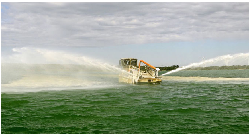
Fig. 4.5 Distribution of lime suspension in Lake Burghammer using a Swedish liming ship (Photo: P. Radke/LMBV)
