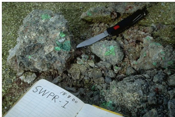
Fig. 5.58 'Evaporate blooms' of nickel precipitates found on the perimeter road
